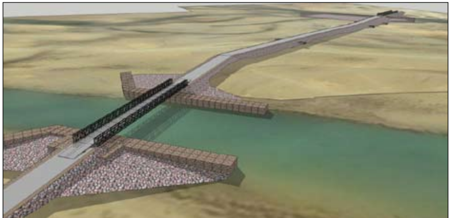
Graphic courtesy of JTF Empire RC-Southwest/West Coordination Cell Plans graphics show the intended scope of Operation Golden Gate, a Regional Command-Southwest combined-joint engineering mission to construct a bridge complex spanning the Helmand River in southwest Afghanistan. The operation design was to improve mobility at the Sabit Qadam Flood Plain Crossing across the river.
