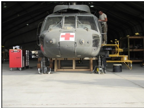
Left: Staff Sgt. Kenneth McDonald, an aircraft mechanic section lead originally from Wilbraham, Mass., completes repairs to a UH-60 MEDEVAC aircraft that is resting on wooden cradles fabricated by the AFSBn-Bagram, 401st Army Field Support Brigade's AC First wood shop.
