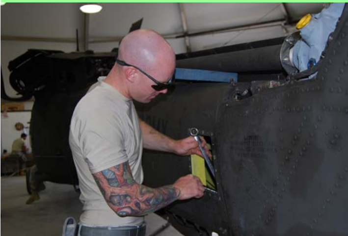
Pictured above: SPC Brandon Cahill performs maintenance on the UH-60 Blackhawk during the Phase Inspection.
