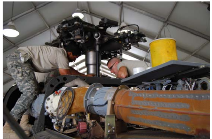
Pictured above: SPC Damon Lappe and SPC Robert Wager work on the main rotor of the UH-60 Blackhawk during the Phase Inspection.
