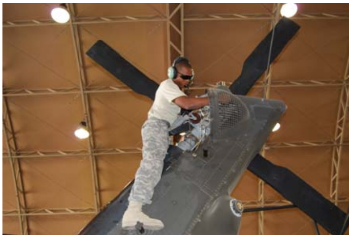
Pictured above: SPC Clifford Coleman performs maintenance on the Tail Rotor section of the Blackhawk during phase maintenance. SPC Coleman's technical skills, work ethic, and attitude have been one of the many keys to success of the Maintenance Platoon.
