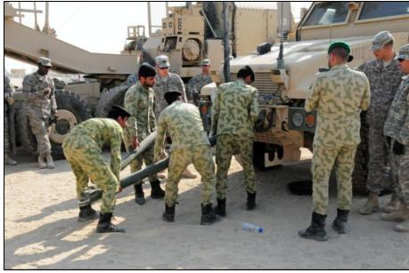
Kuwait National Guardsmen get familiar with hooking up a heavy tow bar to a Mine resistant ambush protected vehicle during the truck rodeo competition, Oct. 9. As part of Operation Steel Sword the truck rodeo is one of five-event exercise designed to foster the exchange ideas and building on the relationship between the Kuwait National Guard and the American Army. (U.S. Army photo by Spc. Michael Gault, Public Affairs, 191st CSSB)
