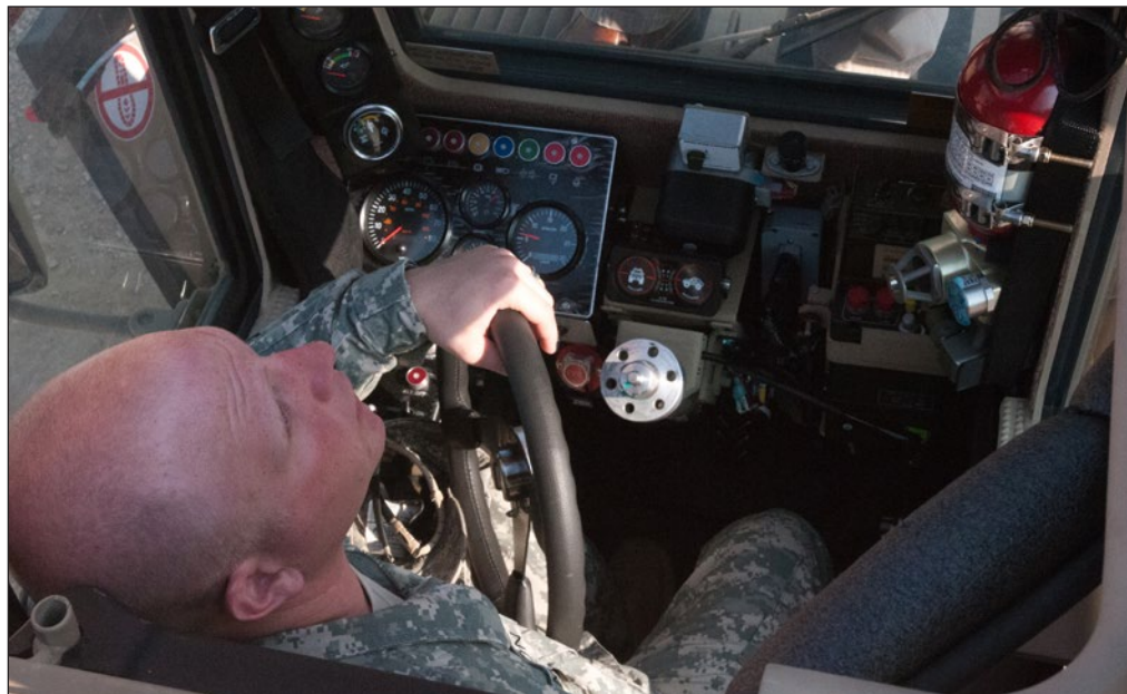
Spc. Matthew Blanton, a combat engineer with 323rd Engineer Company, Spartanburg, S.C., performs a pre-combat check in a Husky Vehicle Mounted Mine Detector, at Fort Bragg, N.C., Aug. 17, 2012. The Husky VMMD is a single operator vehicle that electronically finds improvised explosive devices along the route and marks them with dye. (Photo by Master Sgt. Steve Opet/Army Reserve Command Public Affairs)
